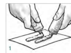
Use the square end of a mixing stick to thoroughly blend the resin and hardener (2).
