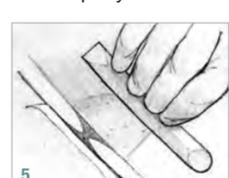
8. Fill the beveled area on the opposite side of the repair with more G/flex 655. Use the side of the mixing stick to feather the edges flush with the surrounding surface and scrape away excess epoxy (5).
