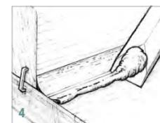
epoxy with the beveled end of the mixing stick before the epoxy gels (4).
