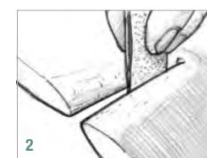
2. Bevel the edges of the crack with a sharp tool to create a 3/8" to 1/2" wide bevel on both sides of the gap and on both sides of the hull including the ends (1).
