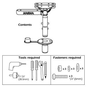
Mirror polished 18-8 stainless steel flush mounted deck socket and post combined with our patented 18-8 stainless steel and hard anodized aluminum "LeveLock" adjustable mount. Allows for quick adjustment. Features a push button/pin lock for instant installation or storage without tools. Sockets include an integral flipup water seal cap.
