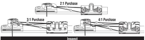
Carefully inspect track and mounting hardware for any signs of loosening, cracks or damage. Inspect end stops to make sure they are secure and that there are no cracks or damage. Arrange control tackle so cars do not hit end stops under load.
