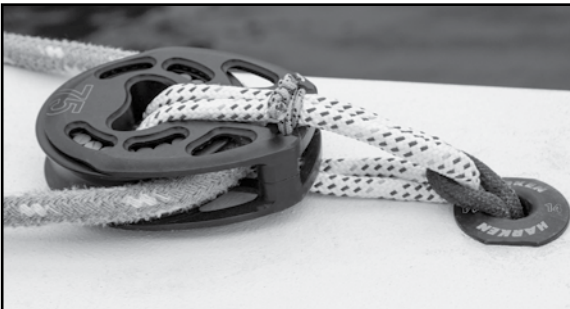
Block attached to soft loop attached to Gizmo padeye kit.
