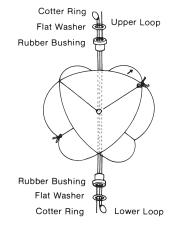
Figure 2. Halyard installation, double loop.
