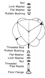
Figure 3. Permanent or hard mounting.
